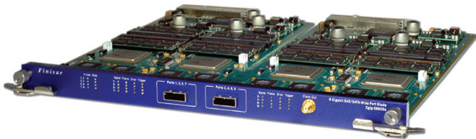
Xgig Platform featuring 6Gb/s Wide Blade
